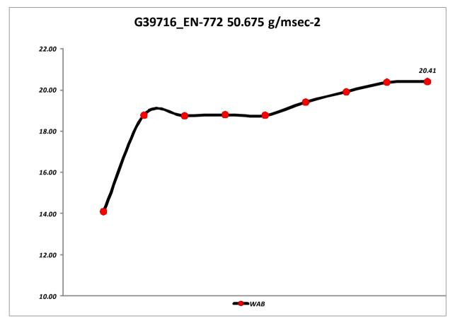
Coefficient of water absorption by capillarity: 50.68 g/m².Sec<sup>-2</sup>
