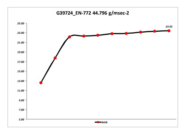
Coefficient of water absorption by capillarity: 44.80 g/m².Sec<sup>-2</sup>
